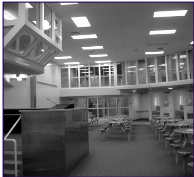
Elevated officer's workstation in a direct supervision housing unit. The elevated area allows the officer to observe both the first floor and second tier from the station.
